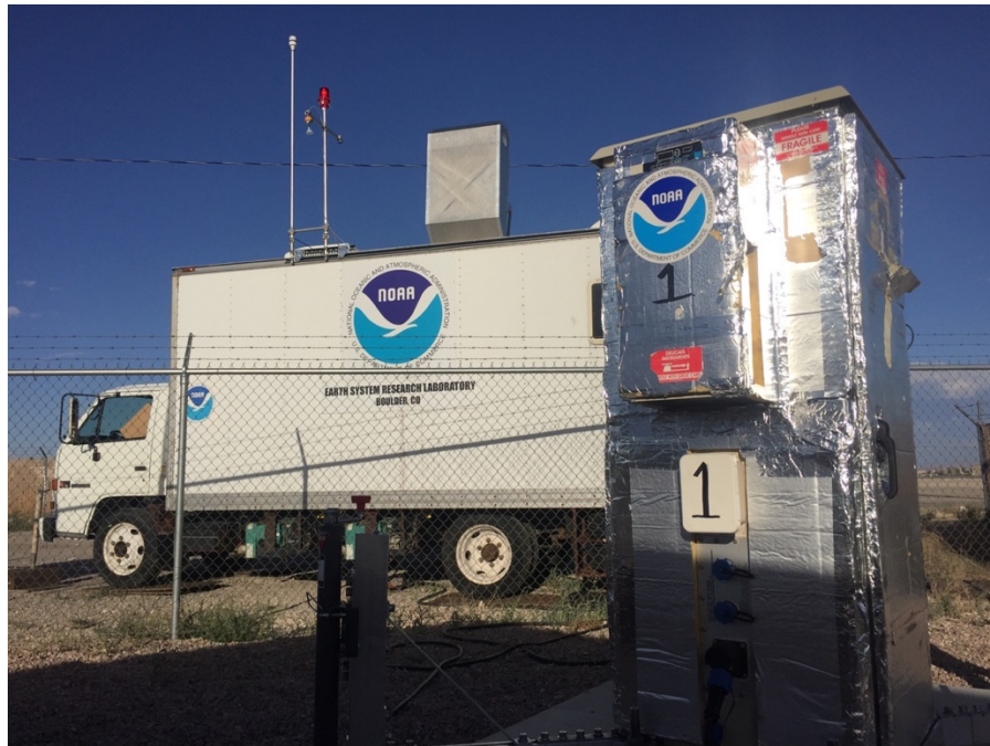
Figure 4-3. The NOAA autonomous micro-Doppler lidar stands on the former RASS pad adjacent to the TOPAZ lidar truck. (photo by A.O. Langford)
